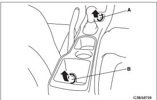
Two accessory sockets are provided in the center console. To use a "plug-in" type accessory, insert it in the socket.
